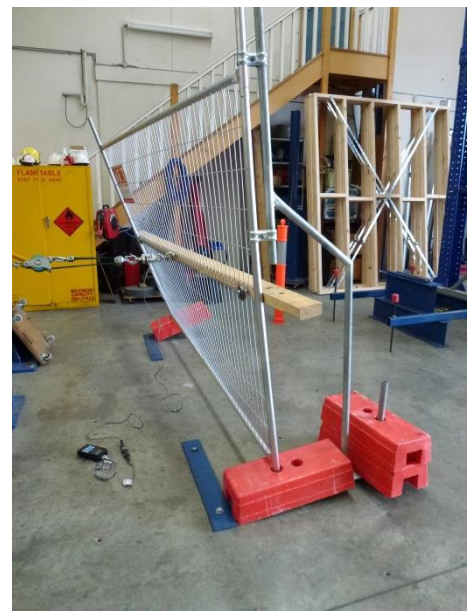
FIG.5 SIMULATED WIND LOAD TEST
